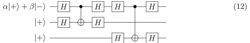
(b) We again attach two ancillary qubits, but instead of wanting to flip the target when the control has value  $|1\rangle$ , we want to flip when the control has value  $|-\rangle$ , so we apply  $H$  only on the control qubits around the CNOT. This results in the following circuit (the input is  $\alpha|+++ \rangle_{ABC} + \beta|--- \rangle_{ABC}$ ).
