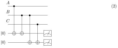
(a) Suppose that an error  $X_{\theta}$  occurred on the qubit A before running the error correction scheme. So the effective circuit with error is
